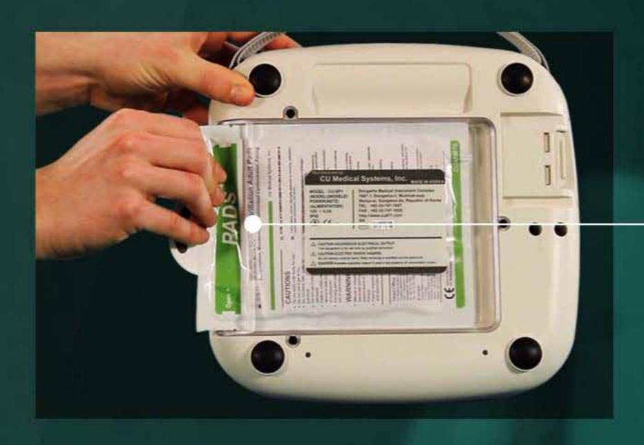
The electrode pads should be firmly in the pad storage compartment on the back of the AED.
