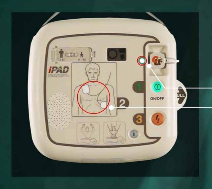
If that light is flashing, check if the pads are correctly connected to the unit. The AED will then give you visual and audible prompts on what to do. Follow these instructions.
