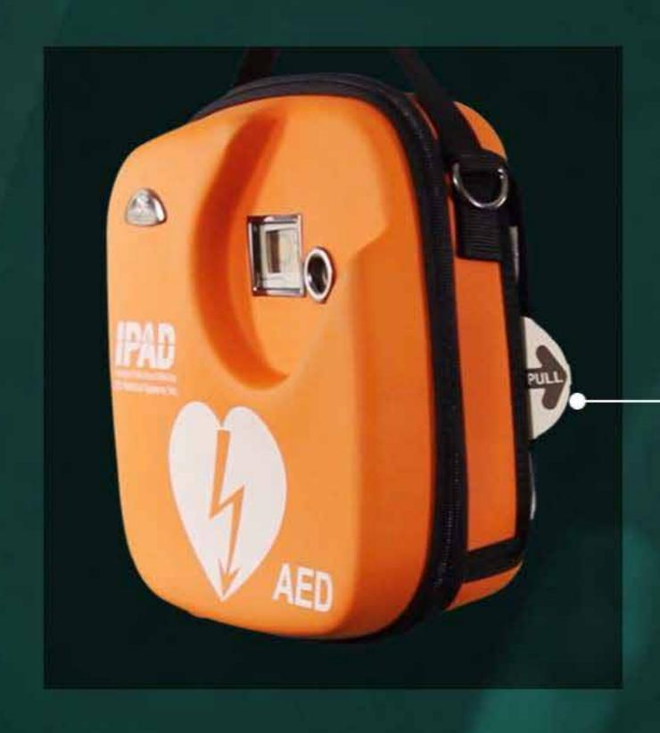
Gently pull the edge of the electrode pads through the slot in the side of the bag, so that the pull tab is visible.
