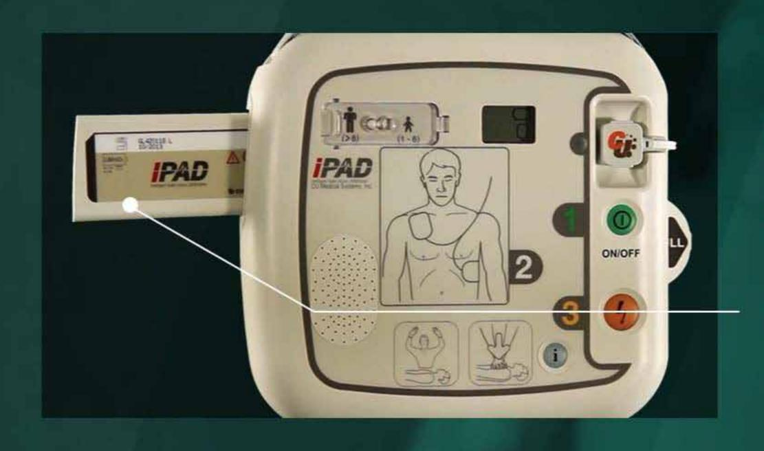
Next, insert the battery pack into the side of the AED in the direction of the arrow on the label.
