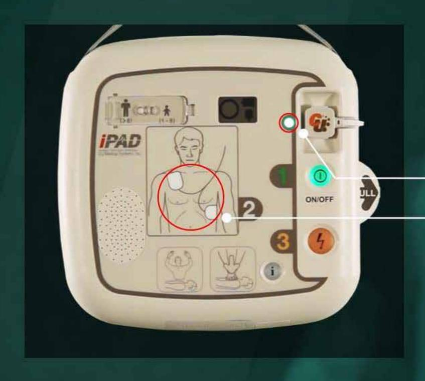
A green light next to the pad's connector will glow only if the electrode pads are properly connected. If the light is constantly lit, the pad connection is good.
