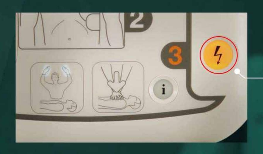
Press the flashing orange shock button.
